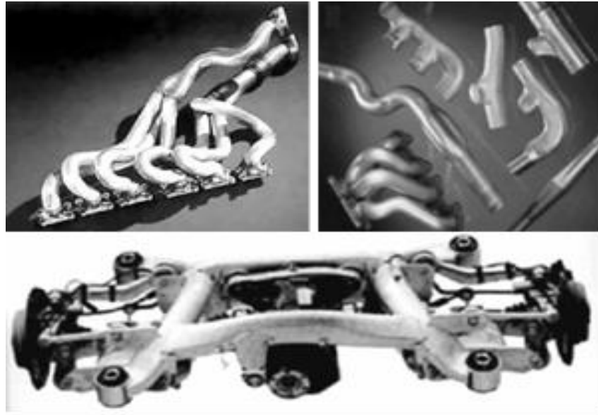
Fig. 5 (i) Exhaust system of BMW M3 and (ii) its elements formed by hydroforming as well as (iii) BMW rear axles with hydroformed components. [20]
