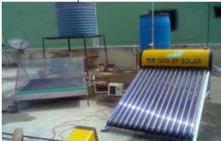
Fig. 9. Experimental setup of solar still coupled with evacuated glass tube [9]
