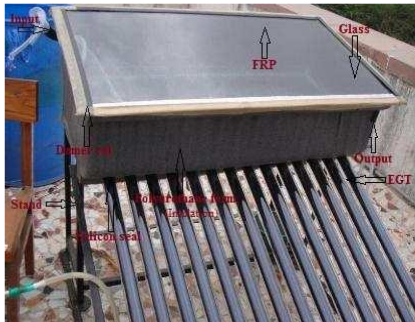
Fig.4. Schematic diagram of solar still coupled with evacuated glass tubes [5]
